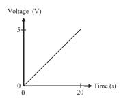
42. A circuit consists of a 500  $\Omega$  resistor connected to a variable voltage source. The voltage is increased linearly from 0 V to 5 V over a period of 20 s, as shown in the graph above. Which of the following graphs corresponds to the power dissipated by the resistor as a function of time?
