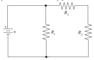
Determine the total power dissipated through the circuit shown above in terms of V,  $R_1$ ,  $R_2$ , and  $R_3$ .
